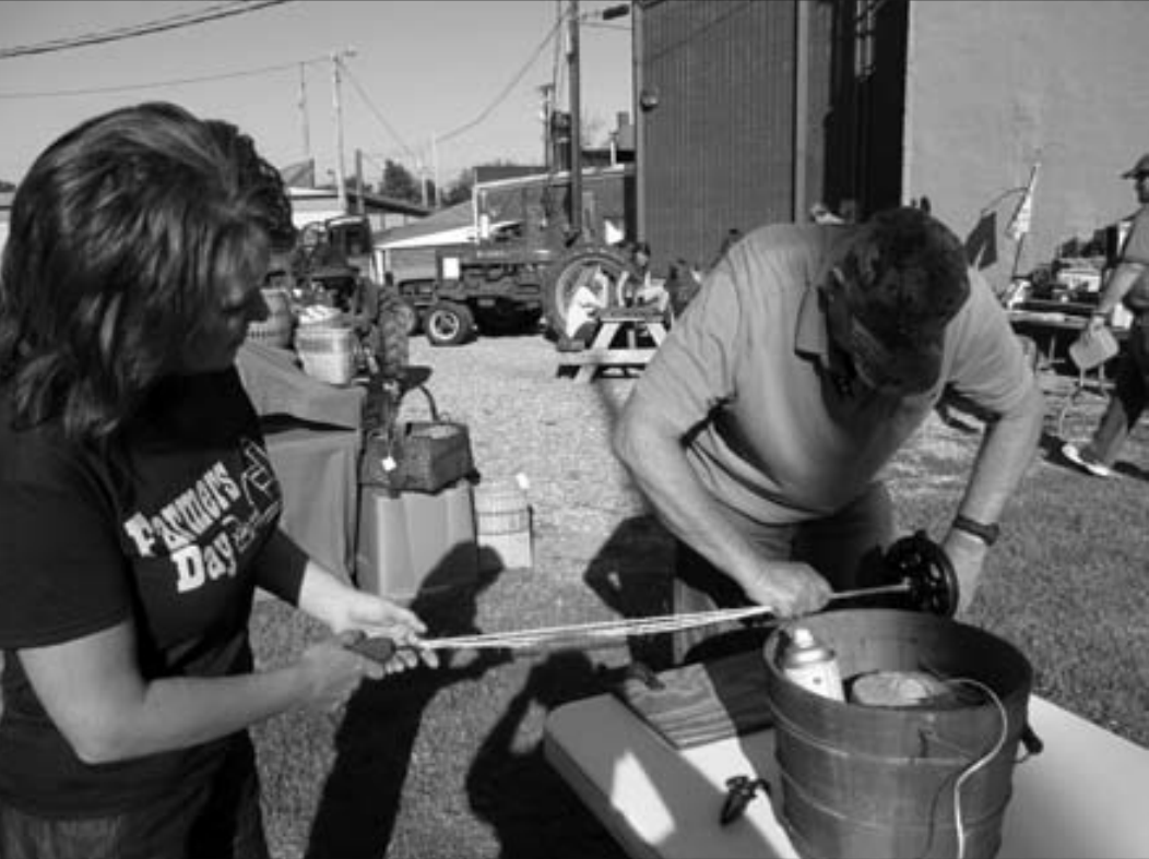
PHOTO BY JASON TRAVIS, THE PRESS Crittenden County resident Clifford Erickson demonstrates the Hawkeye Rope Machine to Deitra Beavers of Farmers Bank. The machine was manufactured around 1900 and helped to make rope out of individual strands of string.
